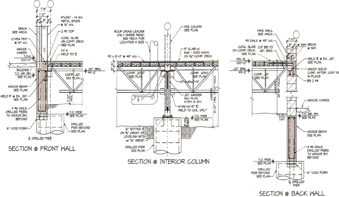
FIGURE 1 DESIGN DETAILS OF THE COMPOSITE STEEL JOISTS
