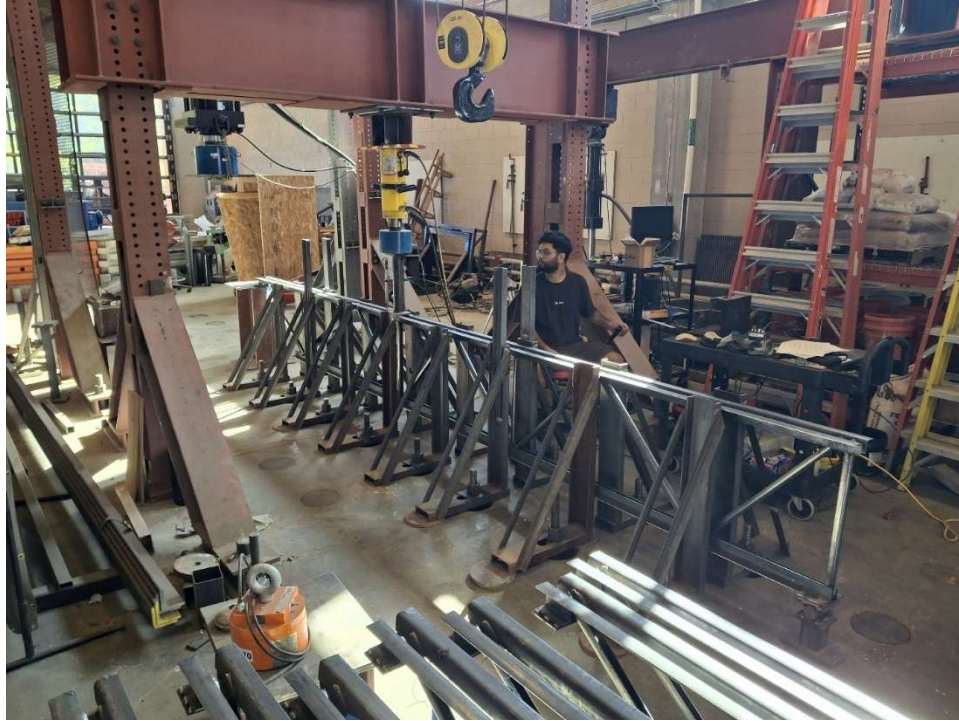
Figure 13. Overall test setup for the batten tests
