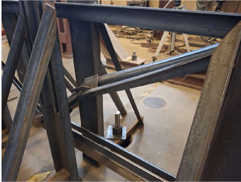
Figure 15. Typical failure mode for specimen group B1 (specimen B1a shown)
