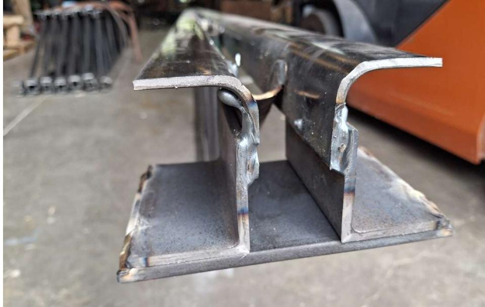
Figure 6: Plate added to seats to prevent splaying
