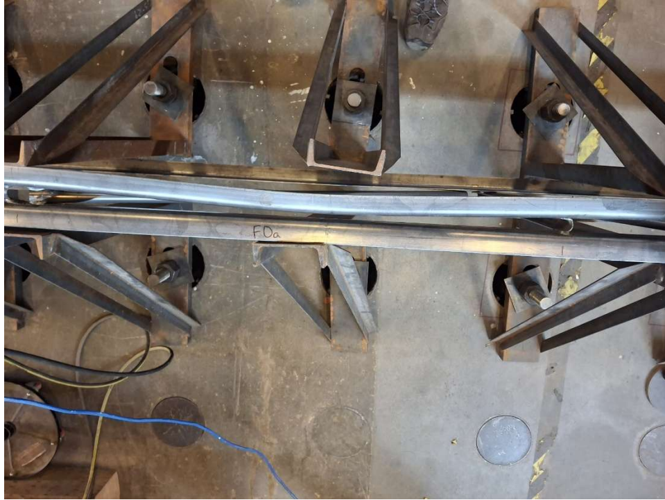
Figure 11. Typical failure mode for specimen group F0 (specimen F0a shown)
