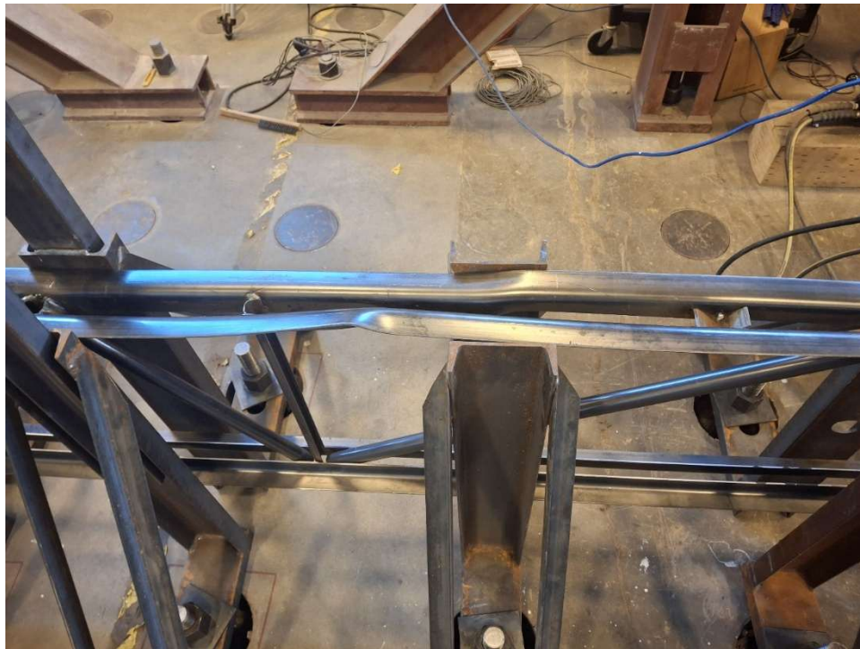
Figure 10. Typical failure mode for filler tests (specimen F1b shown)
