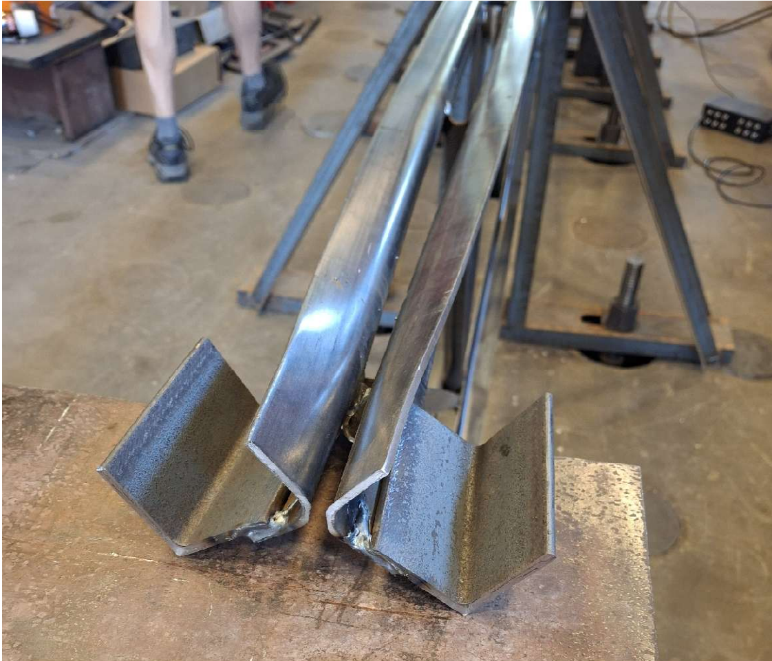
Figure 5: Seat splaying failure of specimen F1a
