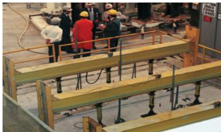
Figure 15. Underwriter's Laboratory fire tests CJ-Series joists.
