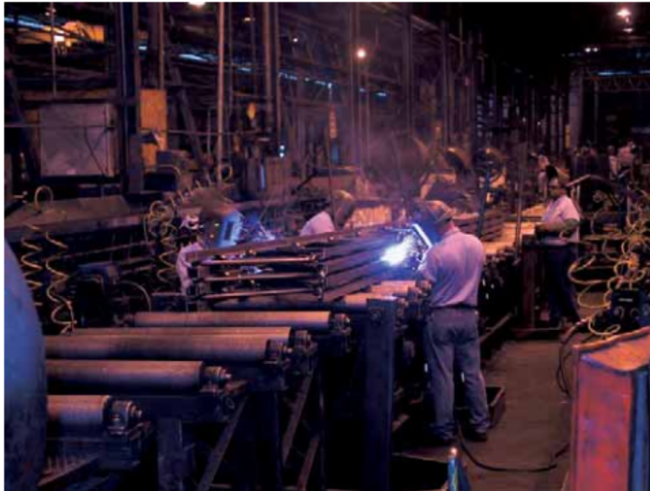
Multiple K-Series Joist being Welded
