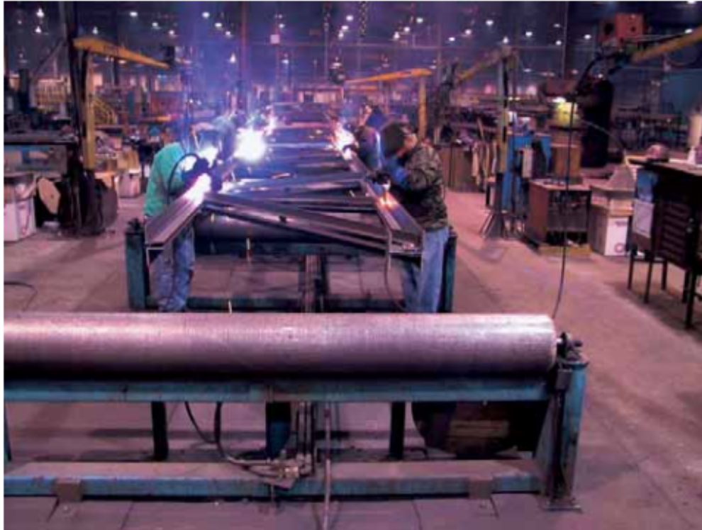
Single Joist Girder being Welded
