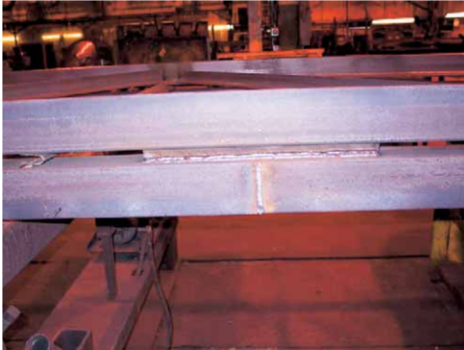
Typical Reinforced Chord Angle Butt Splice
