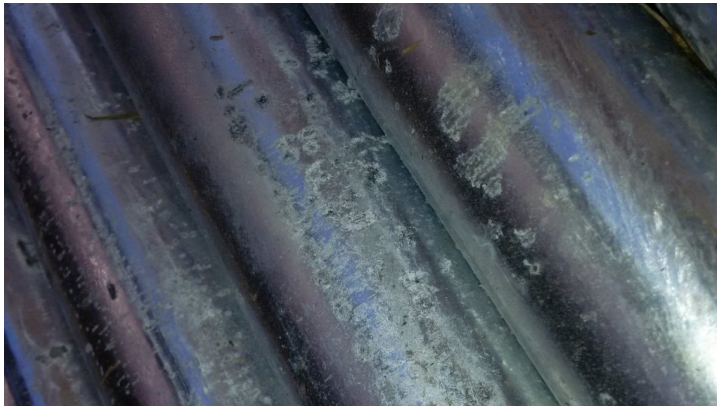
“White Rust” is a different process than “Wet Storage Stain” and you should speak with your electrochemist friends for an explanation
